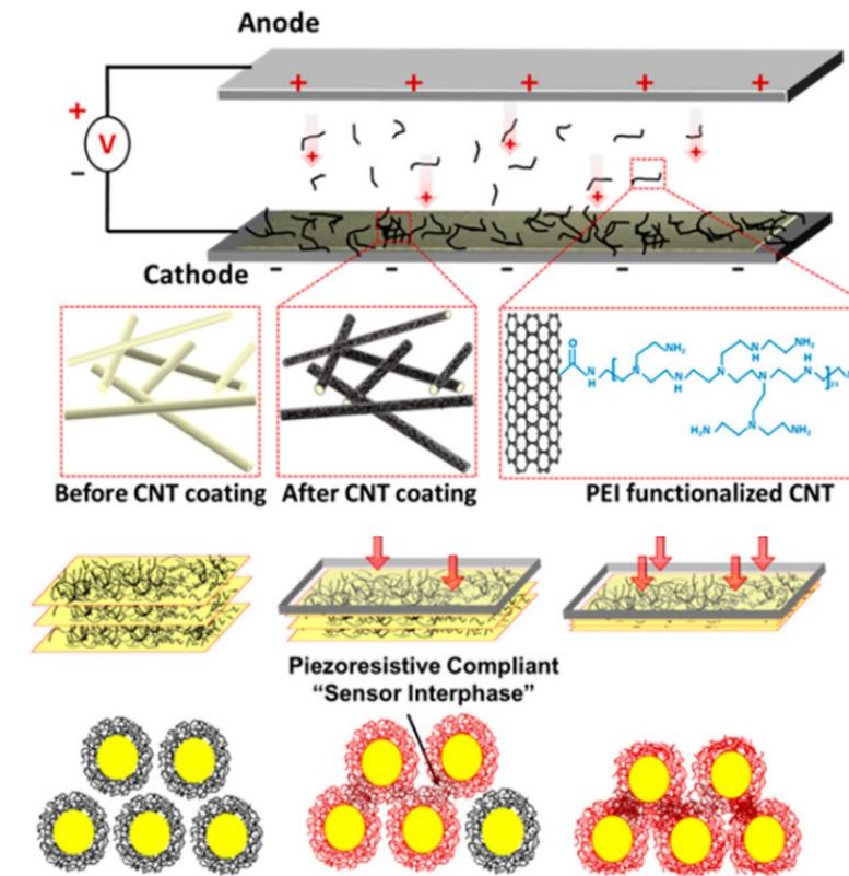
The EPD technique enables the creation of a uniform carbon nanotube-based nanocomposite coating, in the range of 250–750 nm thick, of polyethyleneimine (PEI) functionalized carbon nanotubes on nonconductive fibers. In this work, nonwoven aramid fibers are coated by EPD onto a backing. Electrode followed by film formation onto the fibers creating a conductive network.
