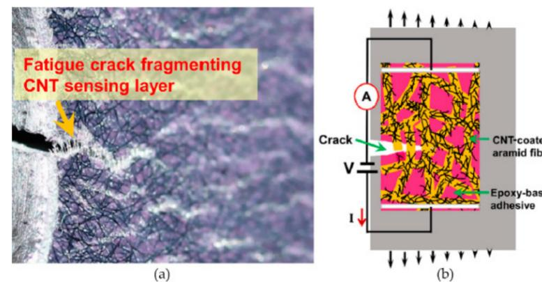
CNT-based thin films have been shown to work well as strain sensors. The small size of the nanotubes, combined with their ability to create electrically conductive networks offers the potential to detect deformation and damage of composite materials in situ and in real time.
